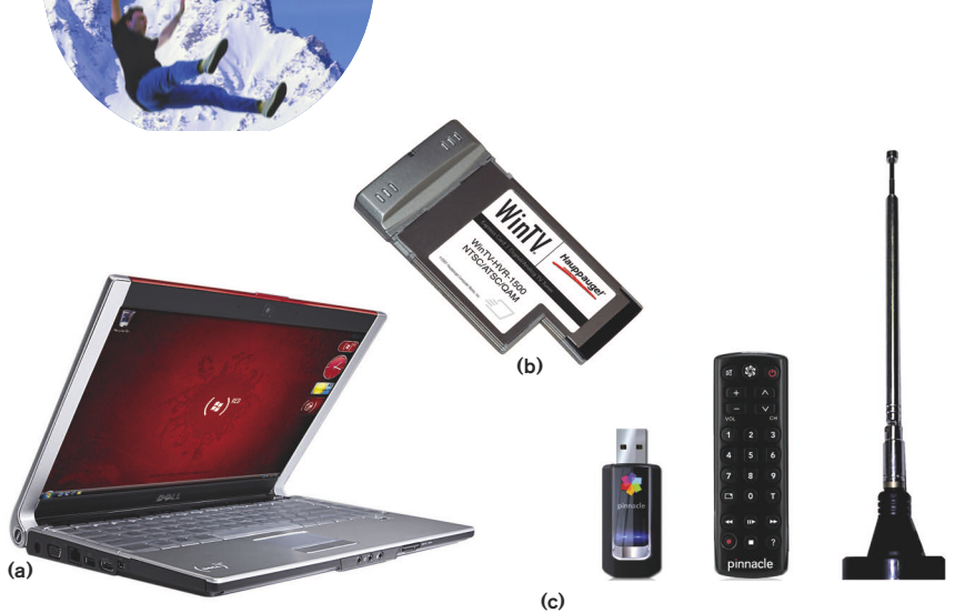
Figure 5 A Dell XPS M1330 laptop (a) became my digital PVR in conjunction with the Media Center application that comes with Windows Vista Ultimate and a Hewlett-Packard-branded version of Hauppauge's HVR-1500 ExpressCard TV tuner (b). I also tried Pinnacle's USB-based PCTV HD mini stick (c), but it created artifact-filled recordings, counterbalancing the unit's robust software suite and integrated "signal booster."
